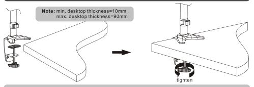
Turn the knob to make clamp fit to desk edge, then secure it tightly.
