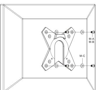
Screw the VESA plate onto the display.
