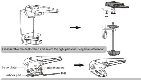
Re-install the base plate with three retained screws, then tighten securely.
