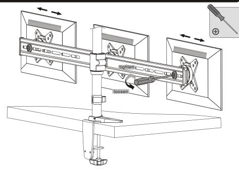
Loosen the screws with a proper screwdriver. Slide the bracket assembly to desired position and then tighten screws to lock the bracket assembly in place.
