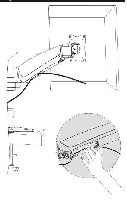
Connect the cables to the display, and press the cable cover inward to route the cables through the space. **Note:** Leave slack in the cable for arm movement.
