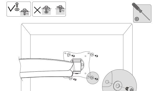
Screw the adapter bracket assembly onto the display.
