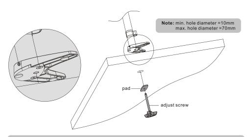
Insert the adjust screw into base plate through the hole. Then using the adjust screw to fix and tighten it securely.
