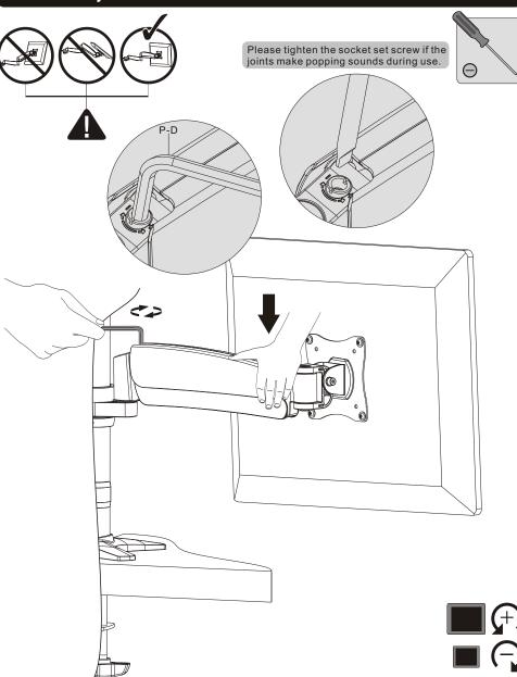
Please keep the forearm level when to adjust pressure. Use a proper Allen key to slightly loosen or tighten the adjustment screw as necessary.
