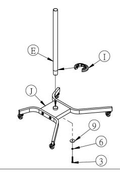
Insert the tube (E) on the pedestal (J), then firmly fix it by screw(3), spring washer (6) and washer (9) from the bottom of pedestal.
