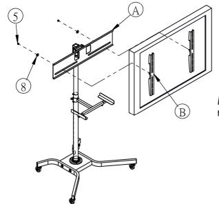
Make sure the mounting arm (B) fix on the TV mounting plate (A) by screw (5) and washer (8).
