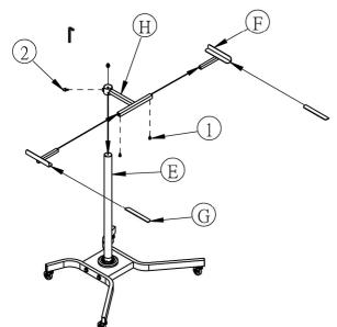
Insert support frame (H) on to tube (E). Insert the movable frame (F) into each side of support frame (H). Put two Velcro (G) on the upper surface of the two frame (F).
