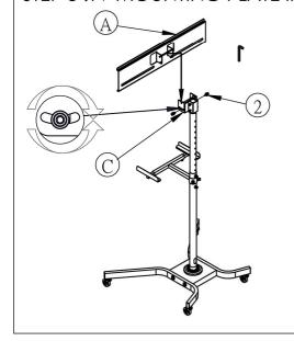
Hang the TV mounting plate (A) onto the joint (C), fixed and adjust the tilting angles with screw (2).
