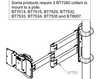
Articulating mounts with the collar icon can be attached to 2 BT7260 collars.
