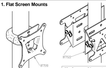
All collar compatible mounts can be mounted back to back. Collar covers cannot be used in this situation.
