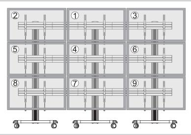
**Note:** The angle of displays are adjusted by the numerical order given.
