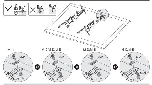
**Note:** Choose the appropriate screws, washers and spacers (if necessary) according to the type of screens.
