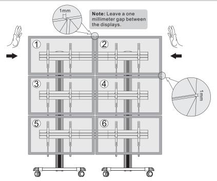
Note: The angle of displays are adjusted by the numerical order given.
