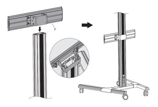
Insert the universal plates to the column along the column rails respectively. **NOTE:** With the arrow pointing upward.
