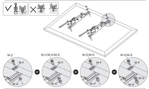
Note: Choose the appropriate screws, washers and spacers (if necessary) according to the type of screens.
