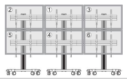
Note: The angle of displays are adjusted by the numerical order given.
