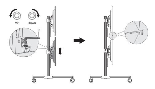
Rotate the adjustment screws as shown in figure to make a one millimeter gap left between the upper and lower displays.
