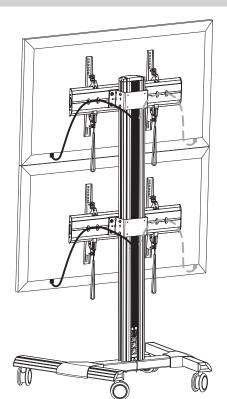
Run the cables through the cable clamps and the rubber strip.
