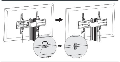
Insert the cable clamps horizontally into the plate slots, then turn the cable clamps to the vertical to secure them.
