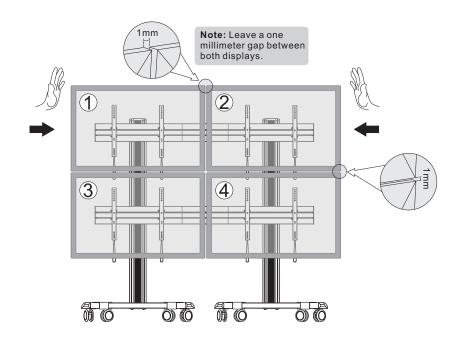
Note: The angle of displays are adjusted by the numerical order given.
