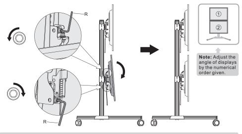
If the displays uptilted, rotate the adjustment screws as shown in figure.
