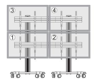
Note: The displays are installed by the numerical order given.
