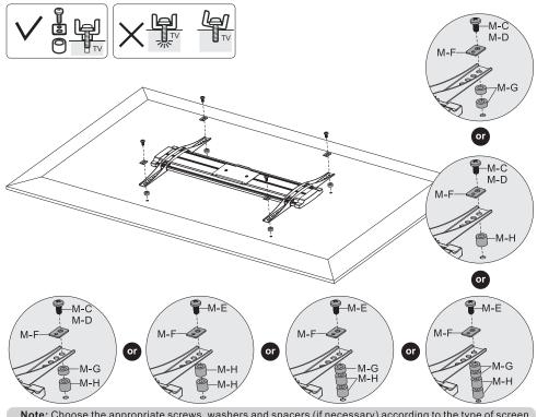
**Note:** Choose the appropriate screws, washers and spacers (if necessary) according to the type of screen. • Screw the adapter brackets onto the display.
