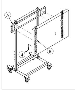
Make sure Mounting arms (B) fixed on the Angle adjustment group (A) by screw(4) well.
