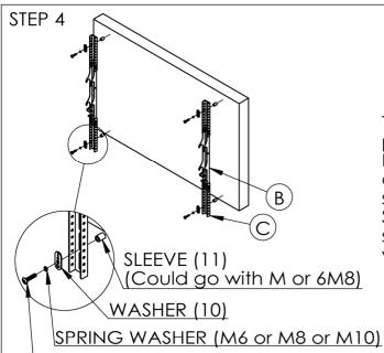
To install Mounting Arms (B) or Extension plate (C) on the back of TV:
