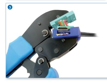
Use the assembly tool to attach the holder to the connector permanently. Fit the cable guides into the the compression guide. Make sure that the wire guides are on the same level and look into the same direction. Press the cable guides into your thumb compression guide until you hear a click. Use you thumb or a rounded non-metal tool for it. Compress the tool. Excessive wiring will be cut off automatically.
