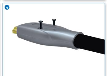
Install the upper half of the metal shell and fix it using the available screws. Be sure to keep the wires away from the screwholes.
